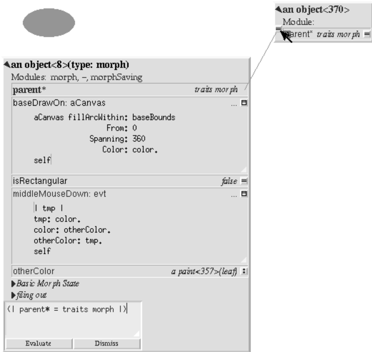
Fig. 7.5: A new traits object has been created to hold behavior to be shared by all instances of the morph. Arrow dragging is being used to make the parent slot of the new morph point to the new traits object.
